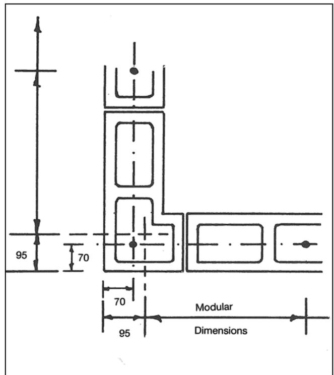
**Figure 7: Positioning corner bar on 150 series**
