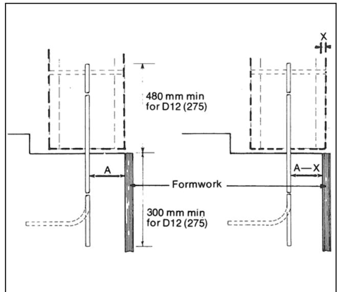
**Figure 6: Position of bar from face of foundation**
