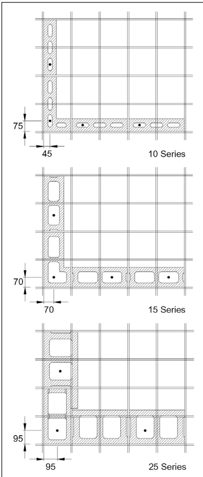
**Figure 2: Modular corner constructions**
