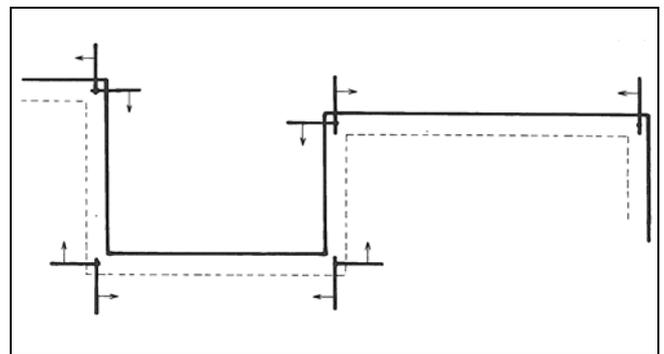
**Figure 4: Work dimensions from each corner**
