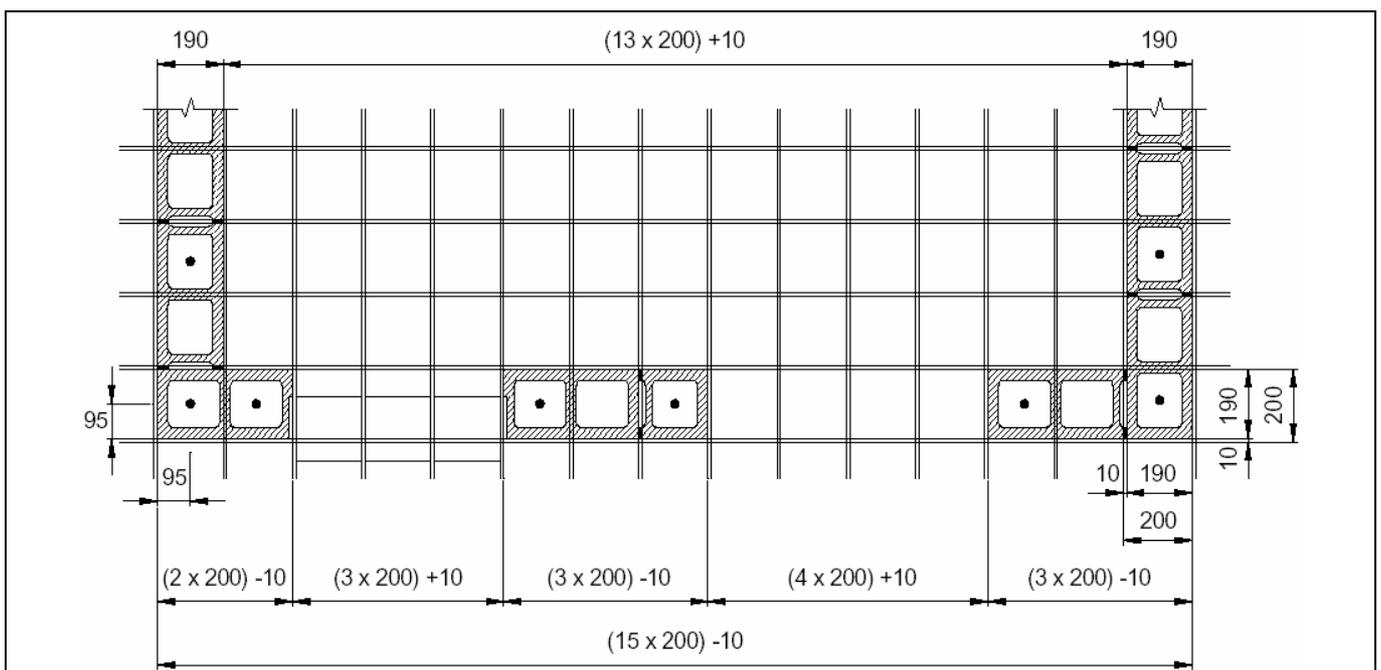
**Figure 1: Planning on the standards concrete masonry grid.**
